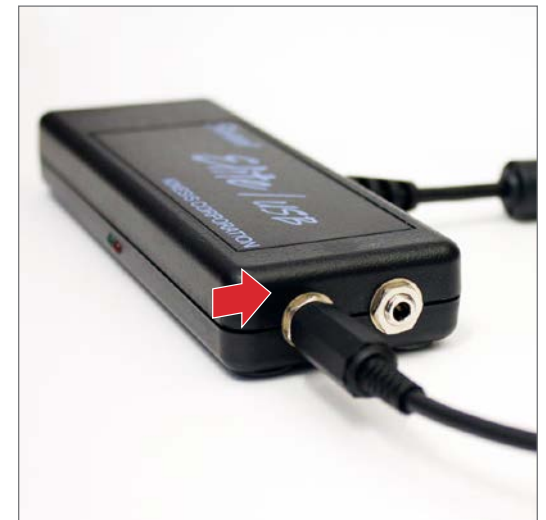
Foot Switch cable plugged into the left socket
