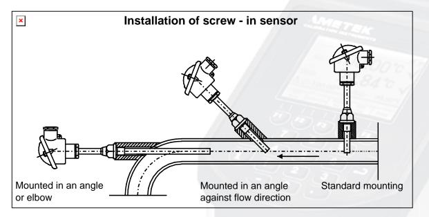
No unique prescriptions are given here as to which mounting should be used for specific measurements. Each individual installation must be evaluated separately. The length of the sensor can be decisive for the way of placing.
