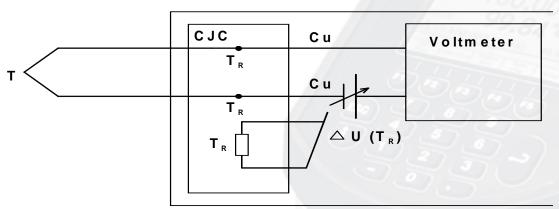
If you have no such instrument available for control of a thermocouple, you may use the following procedure provided that the ambient temperature is known and constant with good approximation:
