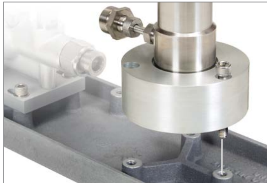
then loosely mount the column.
