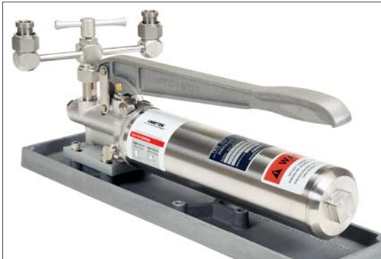
Configuration for comparator testing
