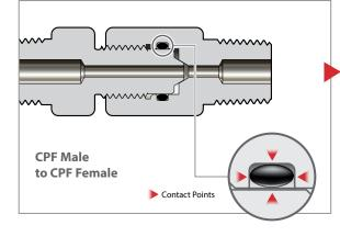
**CPF to CPF O-Ring Seal** Finger-tight up to 10000 PSI/ 700 bar/70 MPa (-20°C to 50°C )
