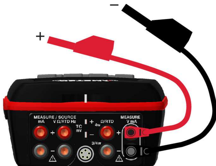
Figure 13 mA current measurement connection (upper window)
