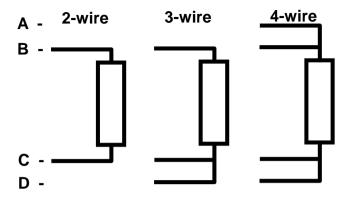
See section 10.0; Technical specifications for supported types of RTDs. The calibrator accepts 2-, 3-, and 4-wire inputs, with the 4-wire input being the most accurate.
