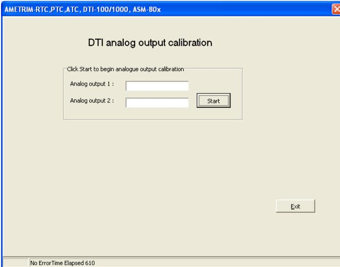
After entering the DTI analog output adjustment window, press “Start” to begin the adjustment procedure.
