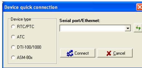
The displayed device types on the left depend on the method and type of comport selected.
