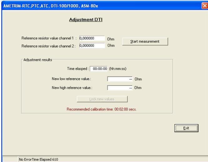
Connect the reference resistors to the input channels and enter the resistor values. Press “Start measurement”, wait until the readings for “New low reference value” and “New high reference value” have stabilized (approx. 2 minutes) and press “Lock new values” to stop the measurement. The locked values can now be downloaded to the DTI or cancelled.
