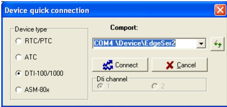
Select “DTI” and “Comport” in the “Device Quick Connect” dialog box and press “Connect”.
