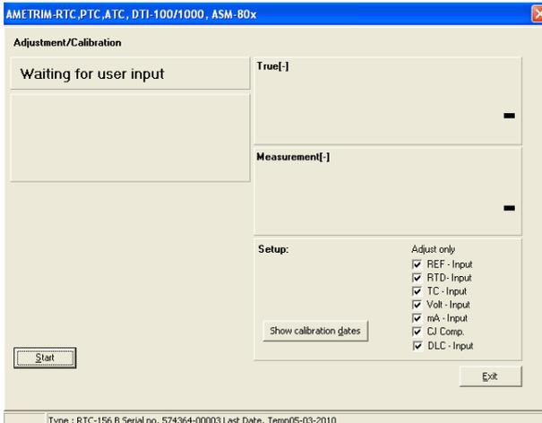
By clicking the Calibration Date button, you can view the last calibration dates for each of the inputs.
