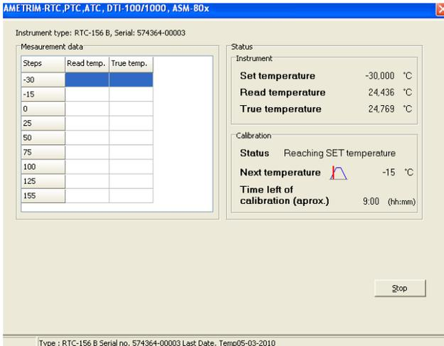
When using the external reference sensor input on the calibrator, or when using a DTI, the calibration and adjustment will now run automatically.
