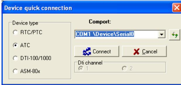
Select “ATC” and “Comport” in the “Device Quick Connect” dialog box and press “Connect”.
