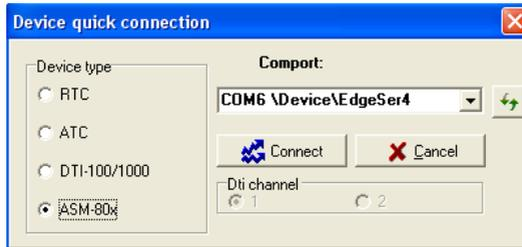
Select “ASM-80x” and “Comport” in the “Device Quick Connect” dialog box and press “Connect”.
