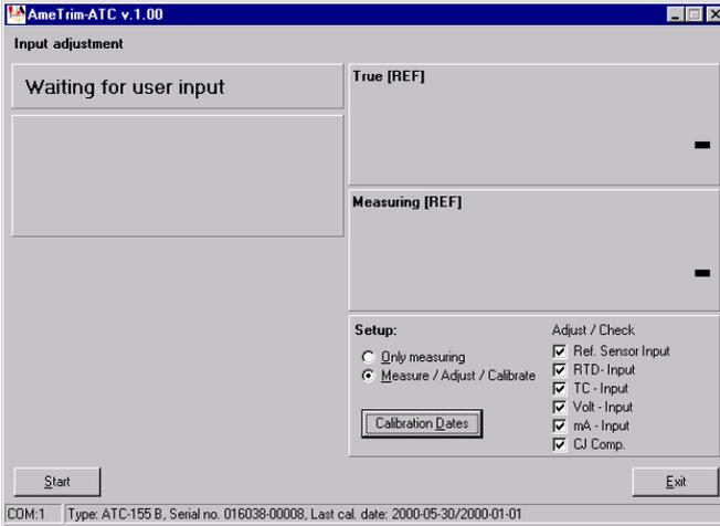
By clicking the Calibration Date button, you can view the last calibration dates for each of the inputs.
