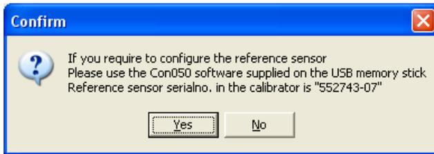
If using the reference sensor on the RTC/PTC scenario, only the Con050 software can be used to configure it.
