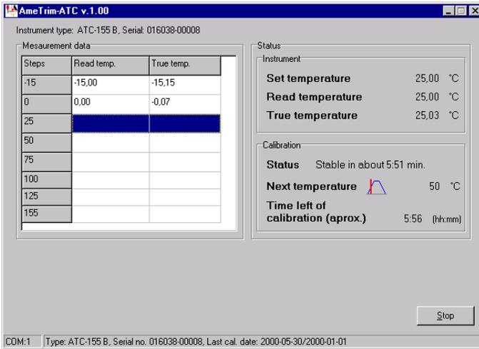
When using the external reference sensor input on the calibrator, or when using a DTI, the calibration and adjustment will now run automatically.
