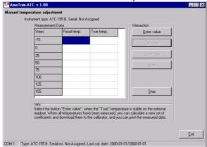
Click OK. The READ temperature measured by the calibrator and the TRUE value are entered in the table.
