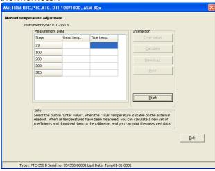
Click OK. The READ temperature measured by the calibrator and the TRUE value are entered in the table.
