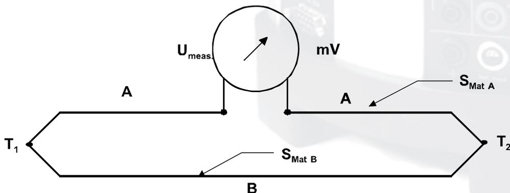
The thermocouple voltage is:  $U_{meas} = (S_{mat A} - S_{mat B}) \cdot (T_2 - T_1)$
