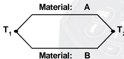
The junctions are normally called soldering points, even though they are most often a welding.
