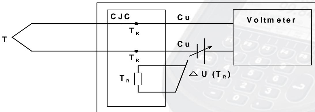
If you have no such instrument available for control of a thermocouple, you may use the following procedure provided that the ambient temperature is known and constant with good approximation:
