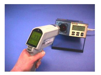
If deviation is recorded, adjust the thermometer accordingly to make the deviation disappear (if possible). After adjustment you need to recalibrate the IR thermometer to control that the adjustment has been successfully carried out. On thermometers where it is not possible to adjust the temperature reading you must record the deviation, to apply correction for the deviation during measurements.
