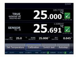
Model B of the RTC is equipped with a built-in accurate measuring circuit for sensor-under-test (input), which enables measurement of virtually any type of temperature sensors including: Resistance thermometers (RTD), thermocouples (TC), transmitters, milliamps (mA), voltage (V) and thermostats.
