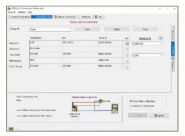
JofraCal is a highly versatile calibration software that is supplied together with the RTC calibrators. The software ensures easy calibration of all kinds of temperature sensors, such as RTD's, thermocouples, transmitters, and thermoswithes. Furthermore, it can be used for pressure calibration i.e. pressure gauges and pressure switches. JofraCal integrates with Jofra calibration instruments. As for temperature calibrators, it is the whole range
