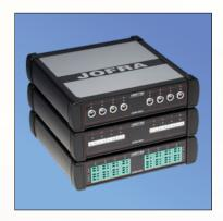
Using the JOFRA RTC series together with the ASM, Advanced Signal Multi-scanner, offers a great time-saving automatic solution to calibrate multiple temperature sensors at the same time. The ASM series is an eight channel scanner controlled by the JOFRACAL software on a PC. Up to 3 ASM units can be stacked to calibrate up to 24 sensors at a time. It can handle signals from 2-, 3- and 4 wire RTD's, thermocouples, transmitters, temperature switches, and voltage.
