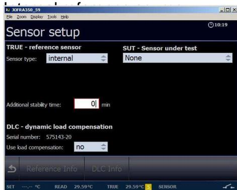
The internal reference sensor will be displayed as the TRUE value on the main screen.
