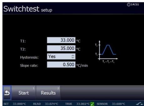
A Switch test setup menu is displayed.
